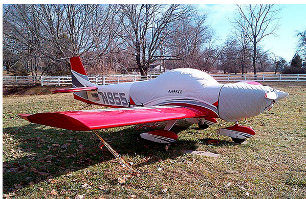
Zenith 601XL Canopy, Prop/Spinner and Insulated Engine Cover
