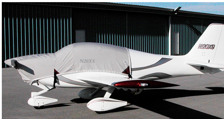
Canopy/Engine and Prop/Spinner Covers (tri-gear model)
