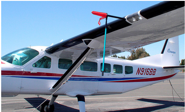
Cessna 208 Caravan Telescoping Pitot (for amphib. models)
