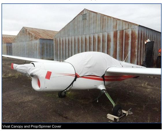
Section 1: Glider Canopy/Cockpit/Fuselage Covers
