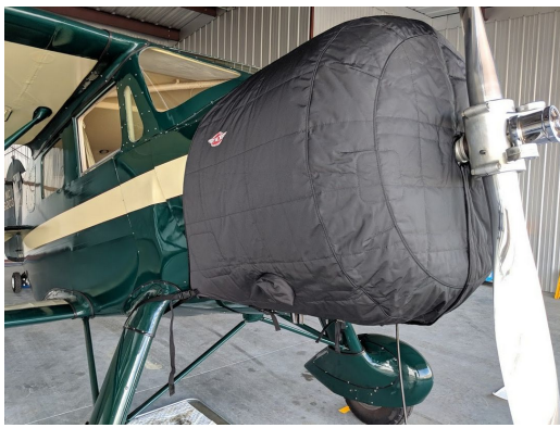
Wacon Cabin Biplane ZQC-6 Insulated Engine Cover
