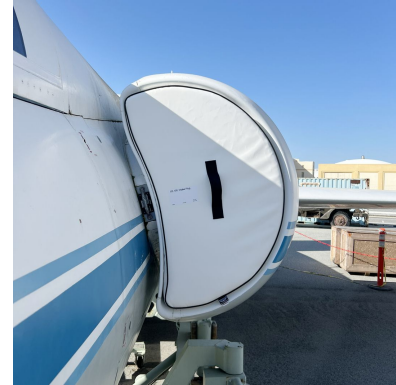
Lockheed U-2 Intake Plugs, test fit plug
