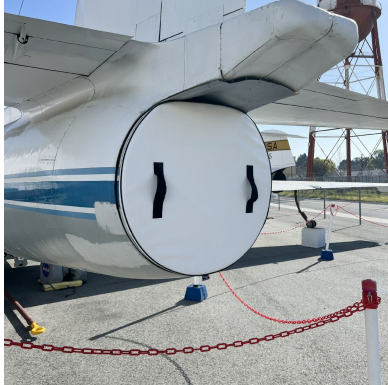
Lockheed U-2 Exhaust Plug, test fit plug
