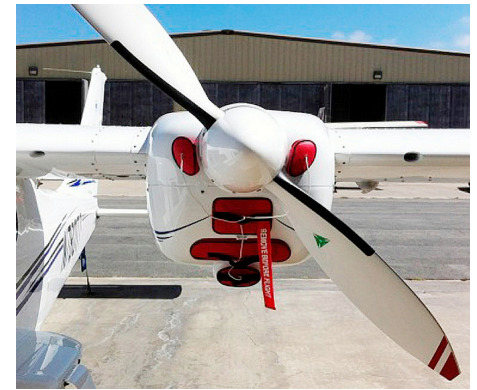
ENGINE PLUGS PREVENT BIRD NEST FOD. Piper Saratoga Engine Cowling Bird's Nest Tecnam P2006T Engine Plugs
