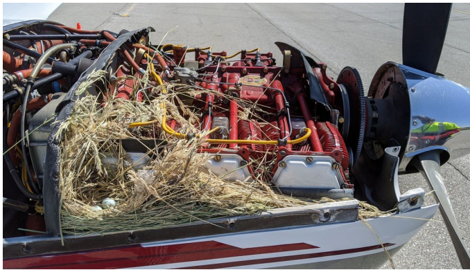
ENGINE PLUGS PREVENT BIRD NEST FOD. Piper Saratoga Engine Cowling Bird's Nest Tecnam P2006T Engine Plugs
