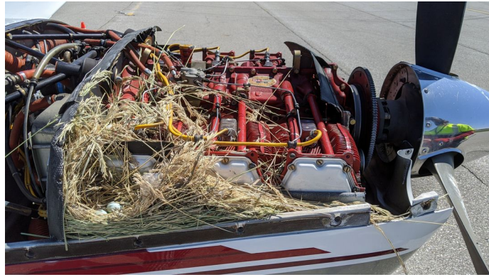
Tecnam P2002 Sierra Engine Plug Set ENGINE PLUGS PREVENT BIRD NEST FOD. Piper Saratoga Engine Cowling Bird's Nest
