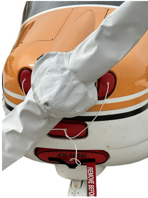
Tecnam P2002 Sierra Engine Plug Set ENGINE PLUGS PREVENT BIRD NEST FOD. Piper Saratoga Engine Cowling Bird's Nest
