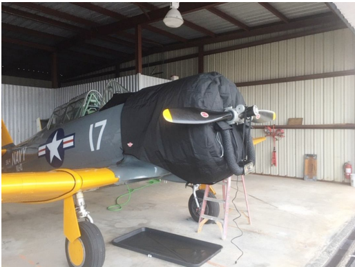
North American SNJ-4 Insulated Engine Cover with Aerotherm Preheater Access Flaps
