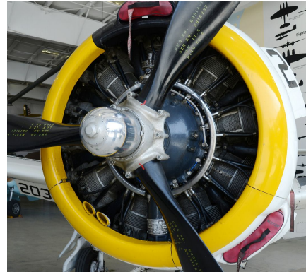
North American T28 Trojan Carb. Air Inlet Plug
