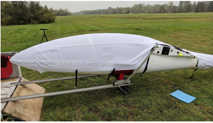
SZD Jantar Canopy/Nose Cover, test fit cover
