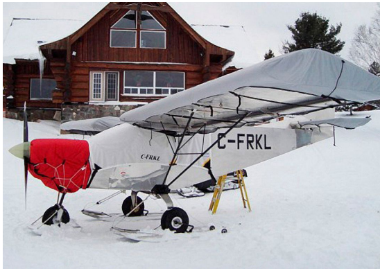
Zenith 801 Insulated Engine, Canopy, Wing & Tail Covers
