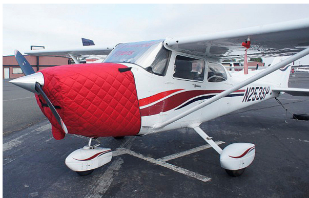
Cessna 172 Insulated Engine Cover, fully enclosed
