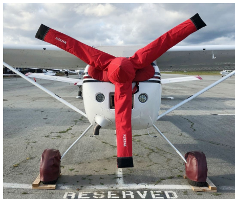
Cessna Skywagon Propellor/Spinner Cover, 3-blade type
