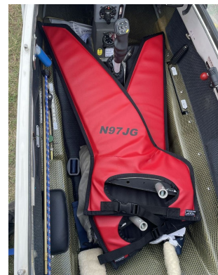
Schempp-Hirth Ventus-2B winglet/wingtip pads
