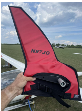
Schempp-Hirth Ventus-2B winglet/wingtip pads
