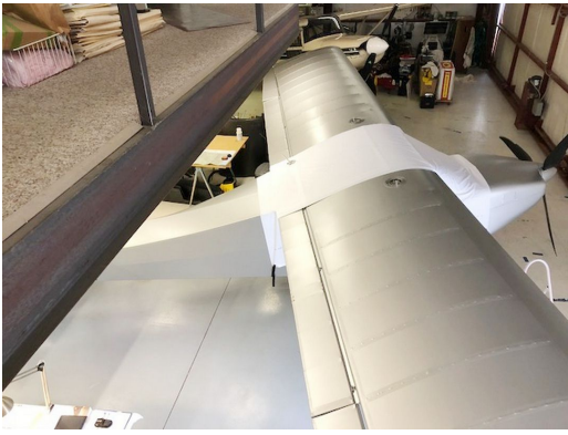
Rans S-20 Canopy Cover, test fit cover
