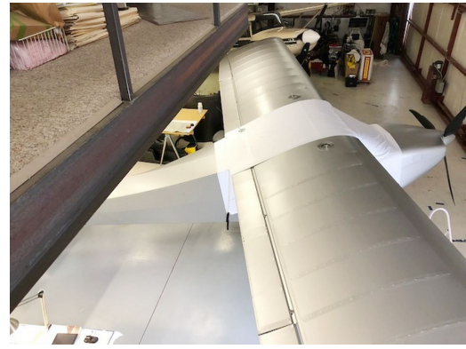
Rans S-20 Canopy Cover, test fit cover
