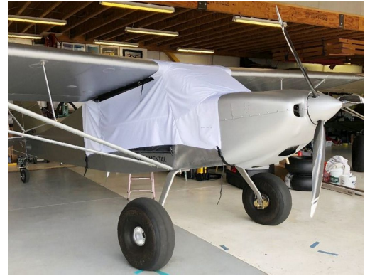
Rans S-20 Canopy Cover, test fit cover
