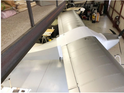
Rans S-20 Canopy Cover, test fit cover
