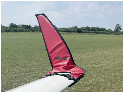
Schempp-Hirth Ventus-2B winglet/wingtip pads
