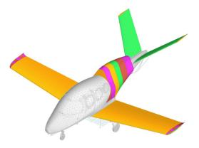
Cirrus SF50 Vision Jet Wing, Aft Fuselage & Stabilizer Covers, 3d Cirrus SF50 Vision Jet Wing, Aft Fuselage & Stabilizer Covers, Model 3d Model
