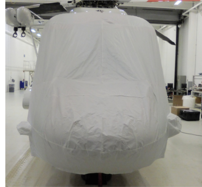
Sikorsky S-92 Windshield/Nose Cover, test fit cover
