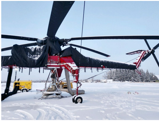
Sikorsky S-64 Skycrane, CH-54 Tarhe Insulated Engine, Rotor Sikorsky S-64 Canopy/Nose, Engine Area, Blade, Rotor, Tail Rotor Hub, Tailboom, Stabilizer & Tail Rotor Covers Sikorsky S-64 Canopy/Nose, Engine Area, Blade, Rotor, Tail Rotor Covers (illustration)
