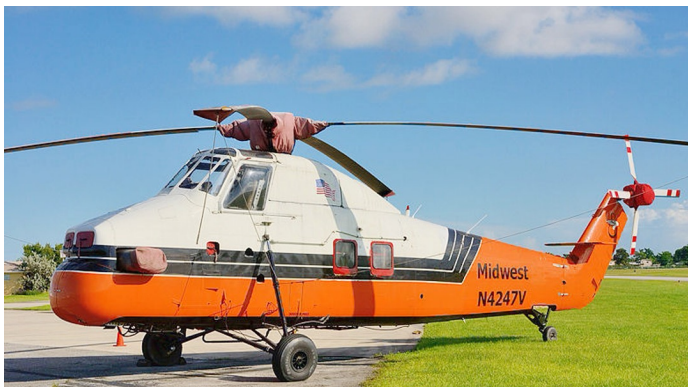
Sikorsky S58T Rotor Hub, Tail Rotor Hub, Engine Plugs, Blade Tie- Downs Sikorsky S58T Travel Cockpit Cover, Engine Plugs and Blade Tie-Downs
