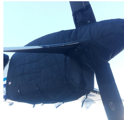
ATR-72-202 Insulated Engine & Prop Hub Covers
