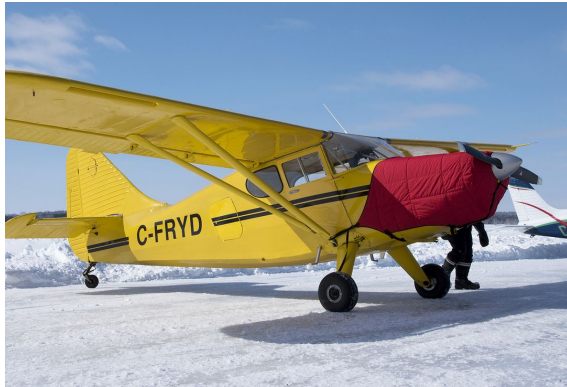
Stinson 108 Insulated Engine Cover, not fully enclosed
