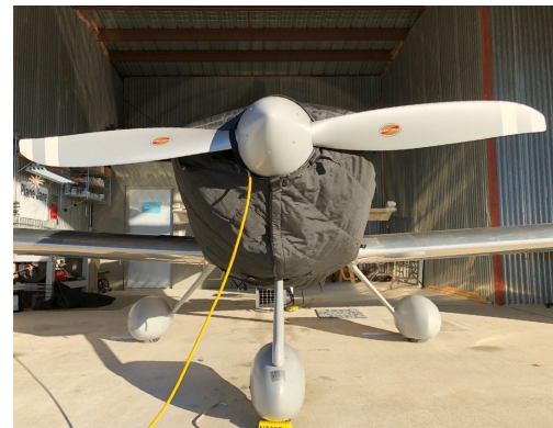
Van's RV-10 Fully Enclosed Insulated Engine Cover
