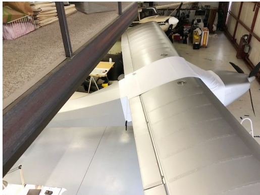
Rans S-20 Canopy Cover, test fit cover
