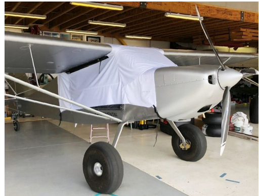
Rans S-20 Canopy Cover, test fit cover
