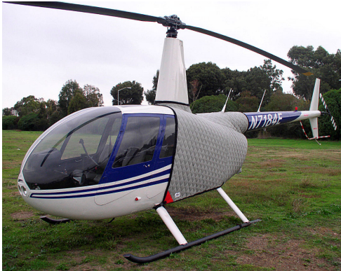
Robinson R-44 Insulated Engine Cover
