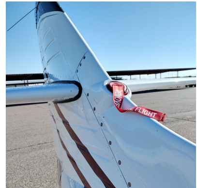
Rockwell Aero Commander 114 Dorsal Inlet Plug
