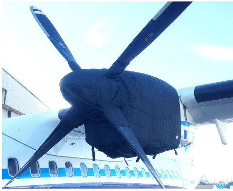
ATR-72-202 Insulated Engine & Prop Hub Covers
