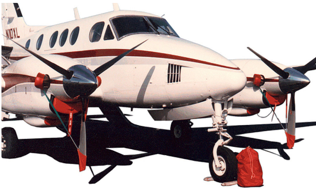
Pitot, Exhaust Covers, Engine Plugs & Prop Ties
