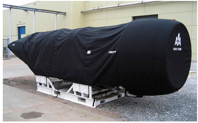
PW JT8D Off-Link Protective Long-term Storage "Rain Cap" Style Engine Cover
