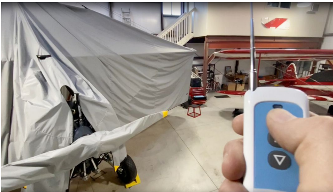
#5: Wireless hoist control.
