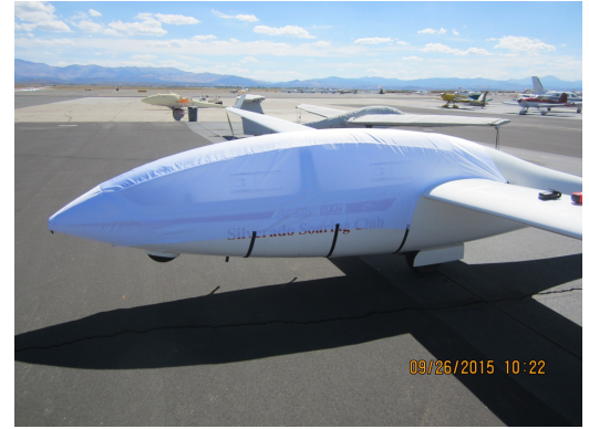
DG-505 Canopy/Nose Cover (test fit cover)
