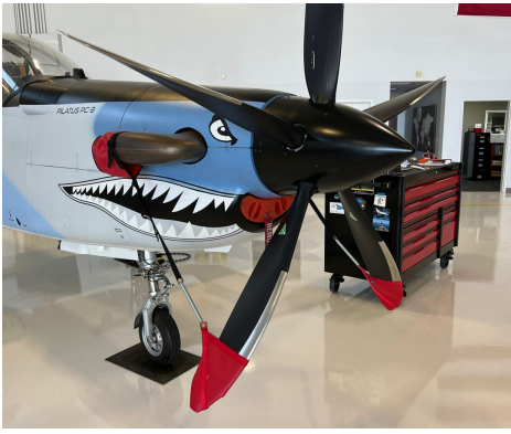
Pilatus PC-9 Prop Ties, Exhaust Covers
