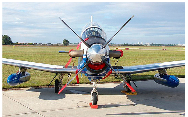
Texan II T6A Engine Inlet Plug, Prop Tie/Exhaust Covers
