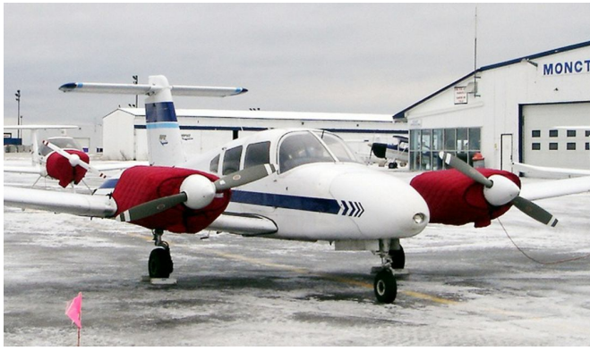
Piper Seminole Insulated Engine Covers
