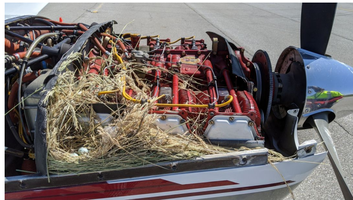
Piper Pawnee PA-25 Engine Inlet Plugs ENGINE PLUGS PREVENT BIRD NEST FOD. Piper Saratoga Engine Cowling Bird's Nest
