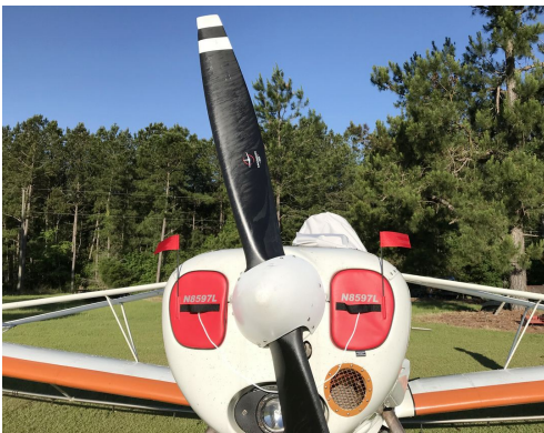
Piper Pawnee PA-25 Engine Inlet Plugs ENGINE PLUGS PREVENT BIRD NEST FOD. Piper Saratoga Engine Cowling Bird's Nest
