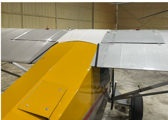
Piper J5A Windshield/Skylight Cover, test fit
