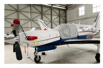
Piper PA-46-500TP Engine Cowling Top Plug
