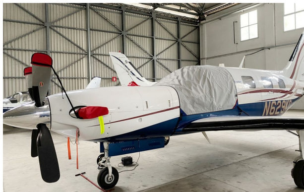
Piper PA-46-500TP Engine Cowling Top Plug
