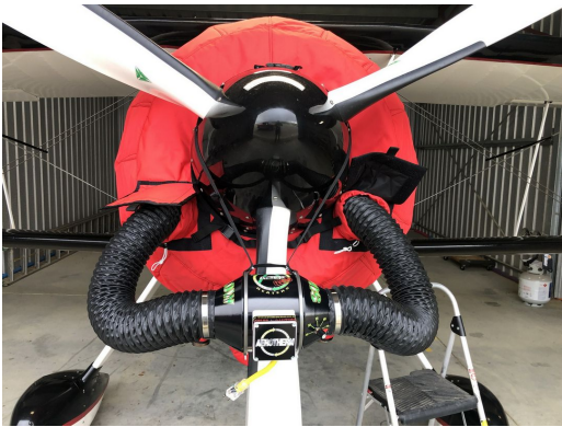
Pitts Model 12 Insulated Engine Cover
