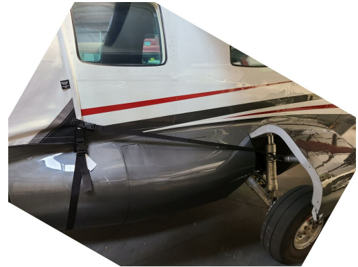
Mitsubishi MU-2 Cockpit/Nose Cover, aft attachment detail
