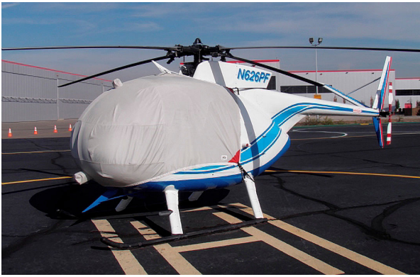
MD500C Bubble Cover with Wire Strike detail
