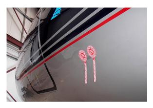
Static Port & Small Inlet/Vent Adhesive Covers: Ideal for Wash Prep and Maintenance
