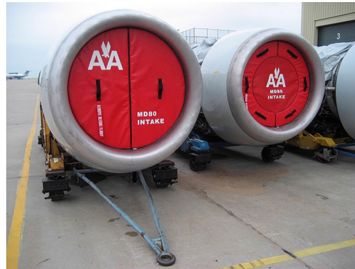
PW JT8D Off-Link Engine Shower Cap Cover Set MD-80 JT8D Intake Plugs, Solid Foam folding type& Mesh Center folding type
