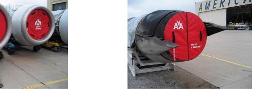
MD-80 JT8D Intake Plugs, Solid Foam folding type& Mesh Center folding type
