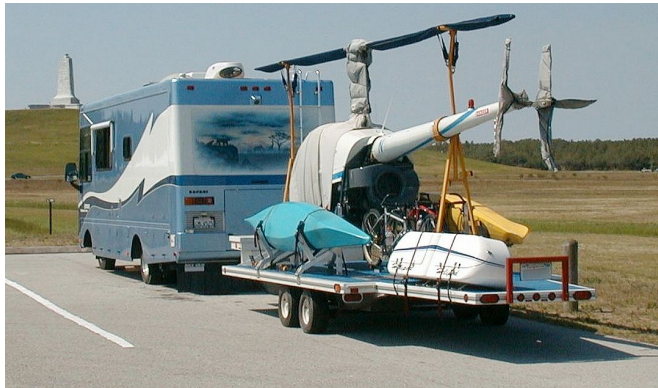
Robinson R-22 Bubble, Rotor Mast, Blades, Tail Rotor & Stabilizer Covers
