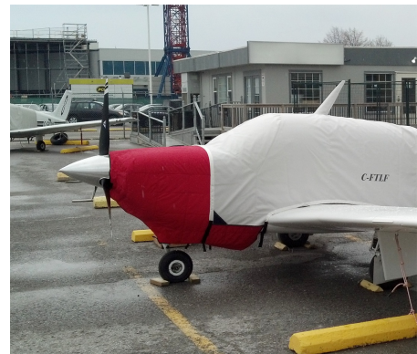
Mooney 201 Insulated Engine Cover, fully enclosed
