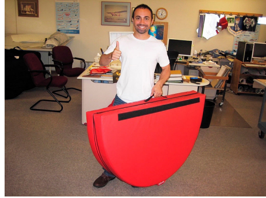
Boeing 737 FOD protection Intake Plug, folding type
