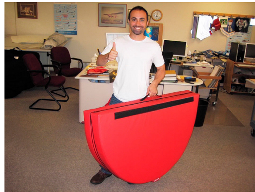
Boeing 737 FOD protection Intake Plug, folding type
