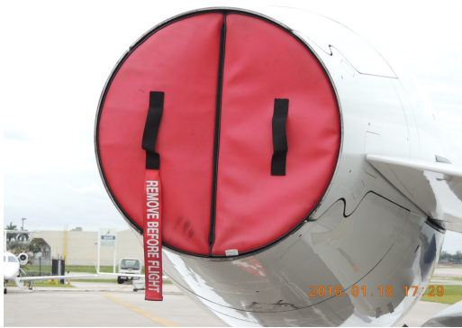
Embraer Legacy 500 Engine Exhaust Plug, folding type
