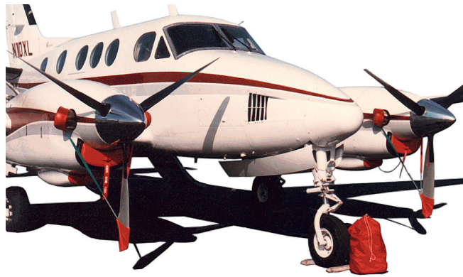
Pitot, Exhaust Covers, Engine Plugs & Prop Ties
