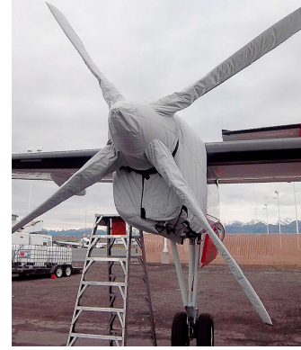
Dash 8 Insulated Engine & Prop Covers
