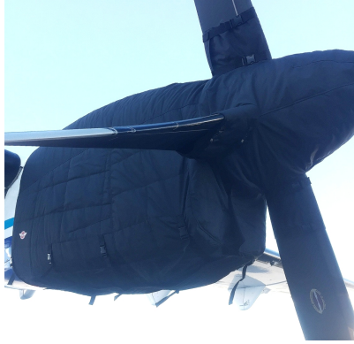
ATR-72-202 Insulated Engine & Prop Hub Covers
