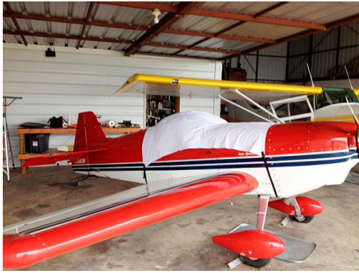
IAC One Design Canopy Cover, test fit cover
