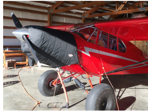
Piper PA-12 Insulated Engine Cover
