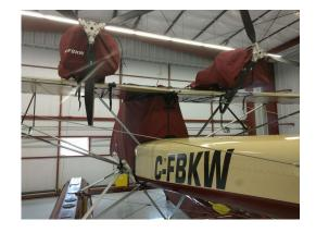
Lockwood AirCam Engine Cover (test fit cover)
