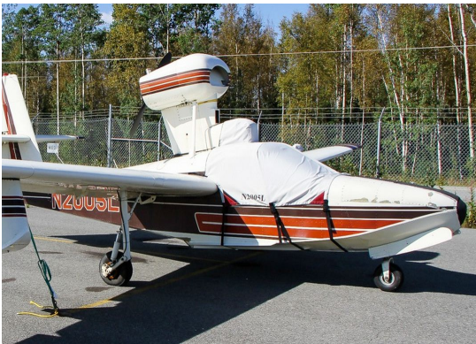
Lake LA4 Canopy Cover with Heater Box
