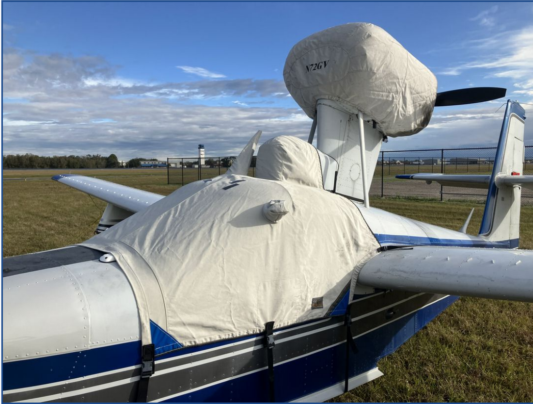
Lake LA-4 Canopy/Heater Box Cover, Engine Cover
